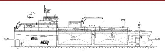
Machinery: **DualFuel-Mecanical Propulsion system** 12V 34DF or equivalent 5400 kW Propulsion power Consumption at 82% MCR 21 t/d
