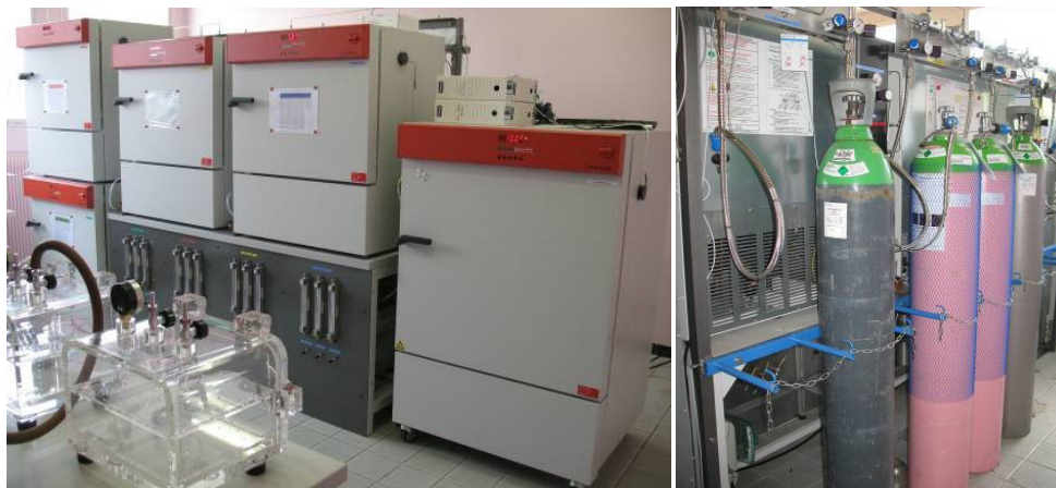
Fig.1: Corrosion simulator - Climatic chambers with their equipment
