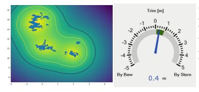
Optimal dynamic trim assists the bridge team in adjusting the ship's trim to the optimum setting, **thereby reducing hull resistance and saving fuel.**
