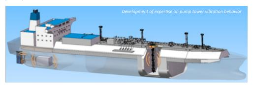
Change in LNGC motorization trends has brought new concerns about the behaviour of the pump tower under vibration. Issues related to these trends have led GTT to further develop its expertise in this domain, in cooperation with Shipyards.
