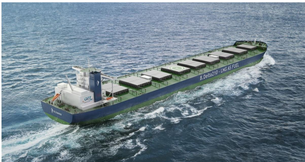
LNG-fuelled Newcastlemax with Mark III membrane tank © Deltamarin – GTT
